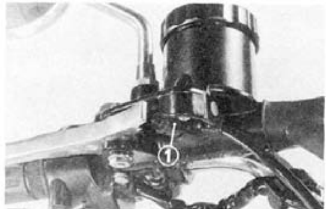
Fig. F2-8 ① front brake switch
