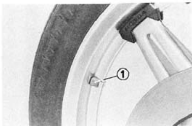
Fig. F2-18 ① Balance weight
