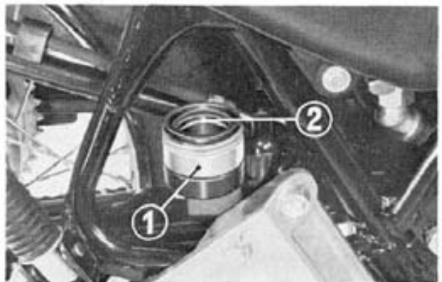
Fig. 47 ① Master cylinder ② Diaphragm
